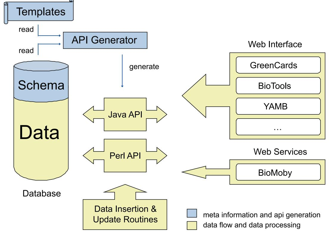
Schematic overview of the GabiPD application structure. The 'API generator' translates the 'Templates' using the database meta-information (shown in blue), generating the database application interface (Java and Perl API). The application logic (shown in yellow), i.e., Web Interface, WebServices and data manipulation routines, interacts with the 'Database' through the database application interface.
